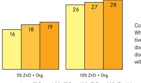
Conclusion: When manufactured effectively microfine zinc oxide does not agglomerate and does not lose performance with time.
